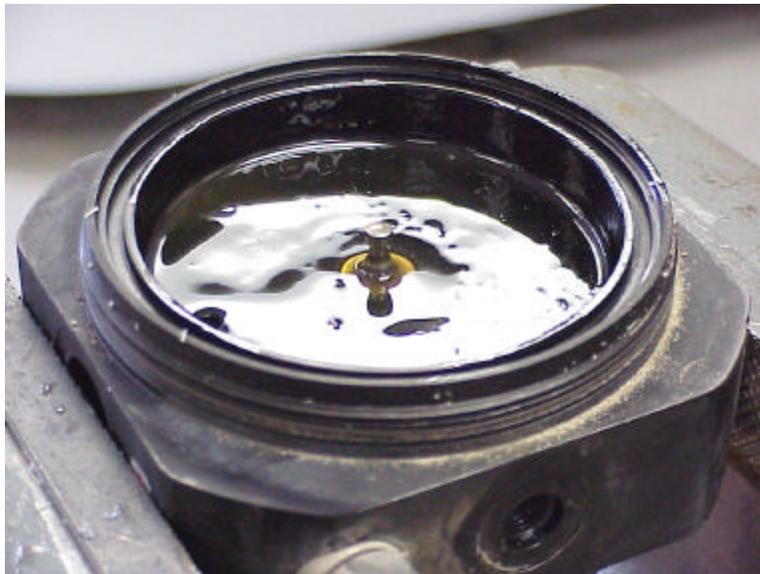
Photo 2 – Oil condensate inside regulator after approximately 35,000 miles.
