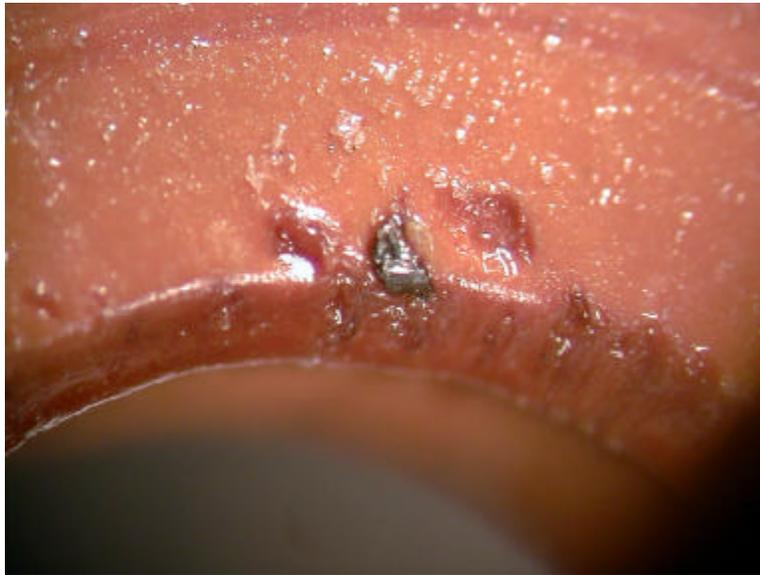
Photo 1 – Microphoto of metallic particulates lodged in valve seat.
